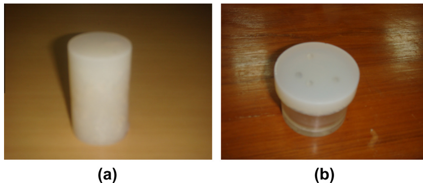
Fig. 1. Photograph of phantom samples (a) mechanical property measurement (b) acoustical property measurement.
